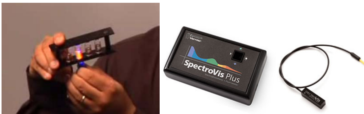
Figure 5. (left) Quantum dots in vials (each vial holds a different size quantum dot) being excited by a blue LED source. (CENCO Scientific) (center) SpectraVis Plus spectrometer. The hole accommodates cuvettes for absorption spectroscopy. (right) A fiber optic accessory can be inserted with its black box like end into the cuvette hole in the spectrometer (aligning the arrows) for emission spectroscopy. Point the fiber optic end at the light source to measure a spectrum.
