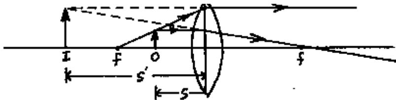
Figure 3: A converging lens with a virtual image.
