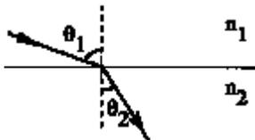
Figure1: A ray of light at an interface
